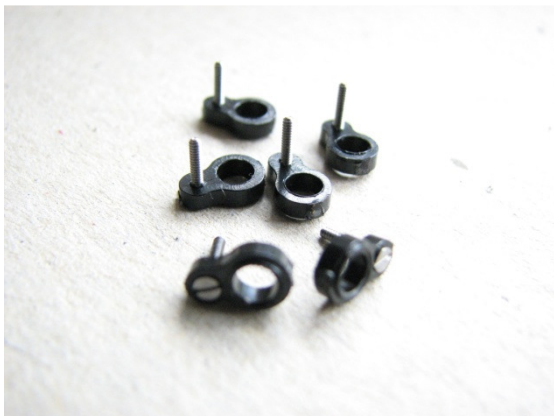
Outside cranks with crankpin pins fitted.
