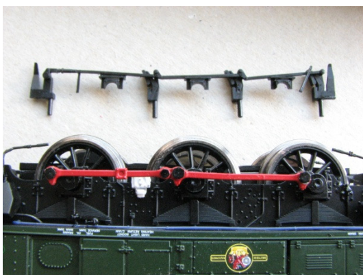
Brake moulding removed.
