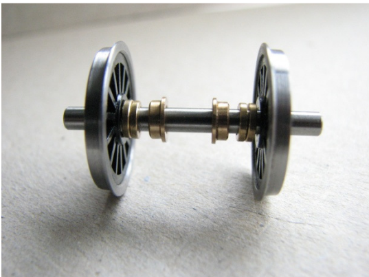
Front wheelset. Note spacing washers and Hornby bearings.
