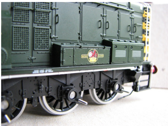
Cranks push fitted to axles. Note they are not fully pushed flush with the axle end yet.
