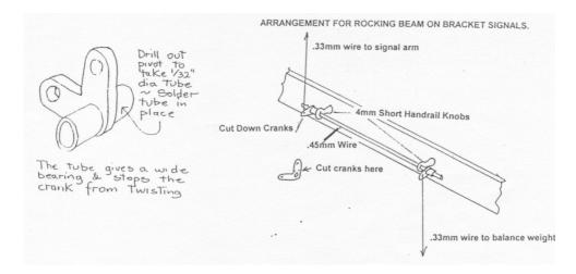
Some signals had rocking beams made up on the edge of the bracket trimmers and our short 4mm scale handrail knobs would be useful for the pivots for these.
