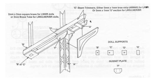
When it comes to the tread and landing these can be made up from individual parts but an etched strip is also available in our range of components. Whichever way you choose it needs to be spaced up from the main trimmer beams by soldering lengths of 1mm x .5mm brass to the underside of it so that the landing is held .5mm away from the beam
